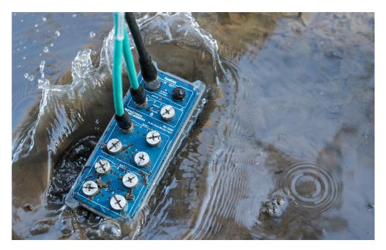
Figure 1. FieldDAQ uses M12 industrial connectors for harsh and vibration-heavy environments.
