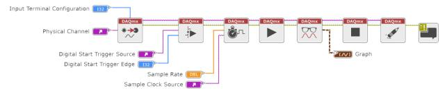
Figure 4. Analog Input Task Designed With the NI-DAQmx Driver and LabVIEW Software
