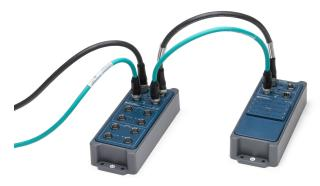
Figure 2. Daisy-Chained FieldDAQ Devices in Line Topology
