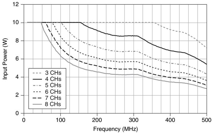
**Figure 2. NI PXIe-2540 Maximum RF Input Power**
