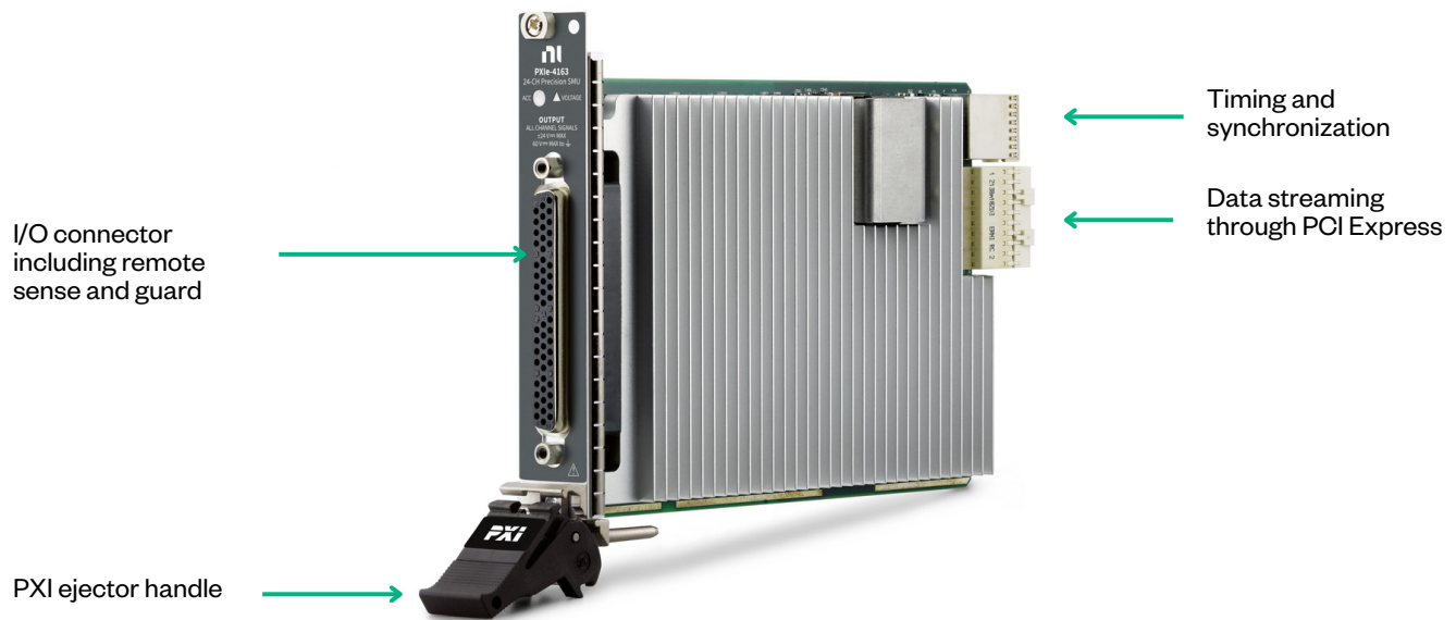
FIGURE 4 Detailed view of the PXIe-4163 SMU
