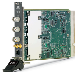
PXI-5922 6 MHz 500 kS/s 2 channels
