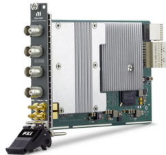
PXIe-5160 500 MHz 2.5 GS/s 2/4 channels
