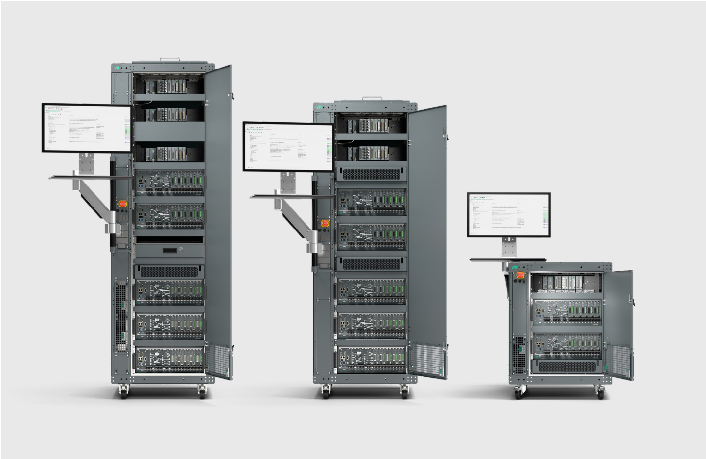
FIGURE 3 ATE Core Configurations come in three different sizes. The 44U provides maximum space, the 38U option is just under two meters tall and can fit through common door heights, and the 15U rack is designed for DUT on top configurations.
