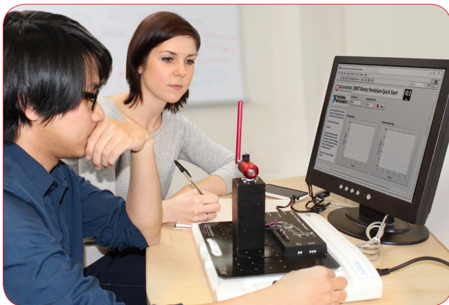
Students learn how to model a pendulum, design and implement controllers to swing up and balance the pendulum in the upright position.
