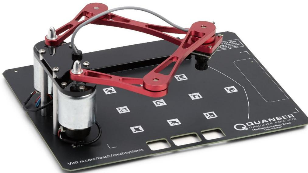
*Figure 1: The Quanser Mechatronic Systems board*
