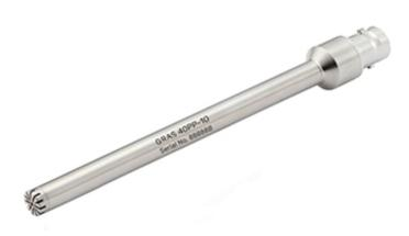
Freq range: 10 Hz to 20 kHz Dyn range: 33 dB(A) to 128 dB Sensitivity: 50 mV/Pa The GRAS 40PP-10 Production-Line Test Microphone is a robust, cost-effective microphone designed for use in the production-line testing of loudspeakers and acoustic transducers. It has a wide frequency range reaching up to 20 kHz and a large dynamic range from <33 dB(A) to 128 dB.
