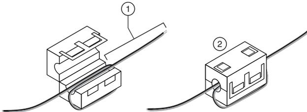
1. Pass the leads through the ferrite twice, leaving 50 mm to 75 mm (2 in. to 3 in.) between the ferrite and the end of the leads.
