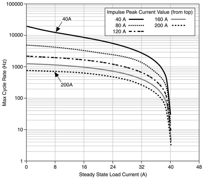
**Figure 3. Maximum Cycle Rate for Multiple Paths Closed**
