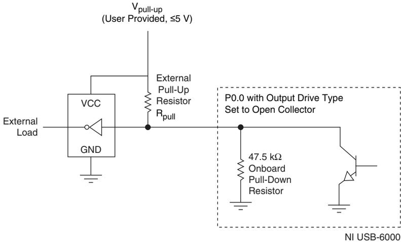
**Note:** Ensure that the current flowing across  $R_{pull}$  does not violate the maximum sinking current specifications (4 mA).
