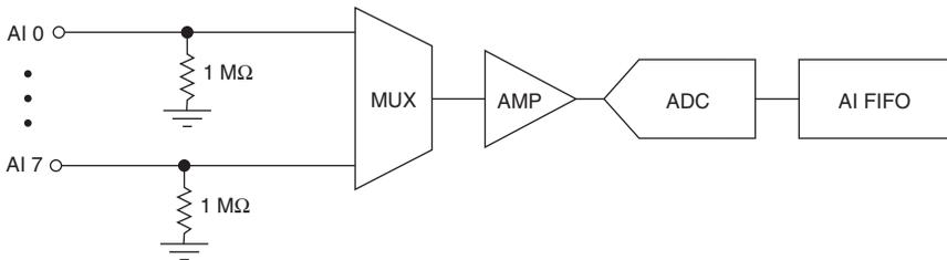
The main blocks featured in the analog input circuitry are as follows:
