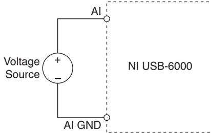
Signals of  $\pm 10$  V at any analog input pin with respect to AI GND are accurately measured. Beyond  $\pm 10$  V, the input signal will begin clipping as shown in Figure 7. Typically, this clipping begins at  $\pm 10.5$  V.
