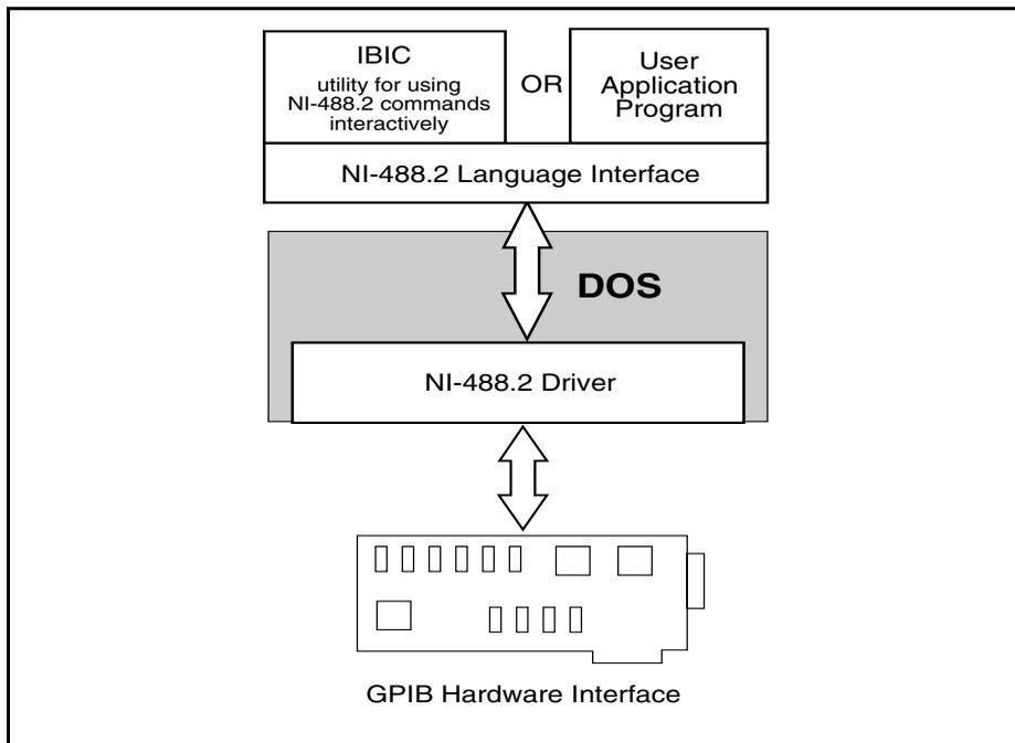
Figure 1-4. How the NI-488.2 Software Works with DOS
