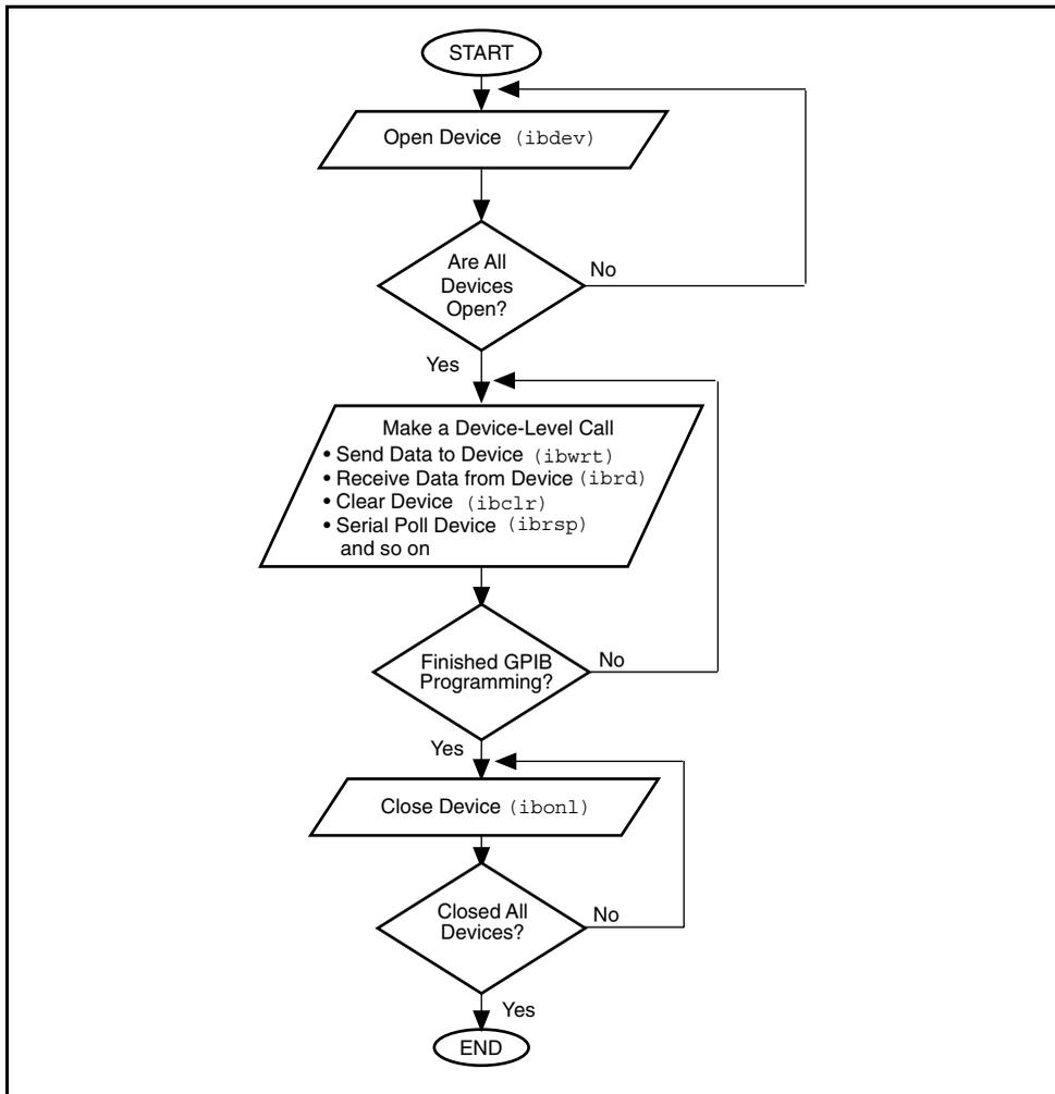
Figure 3-1. General Program Shell Using NI-488 Device Functions
