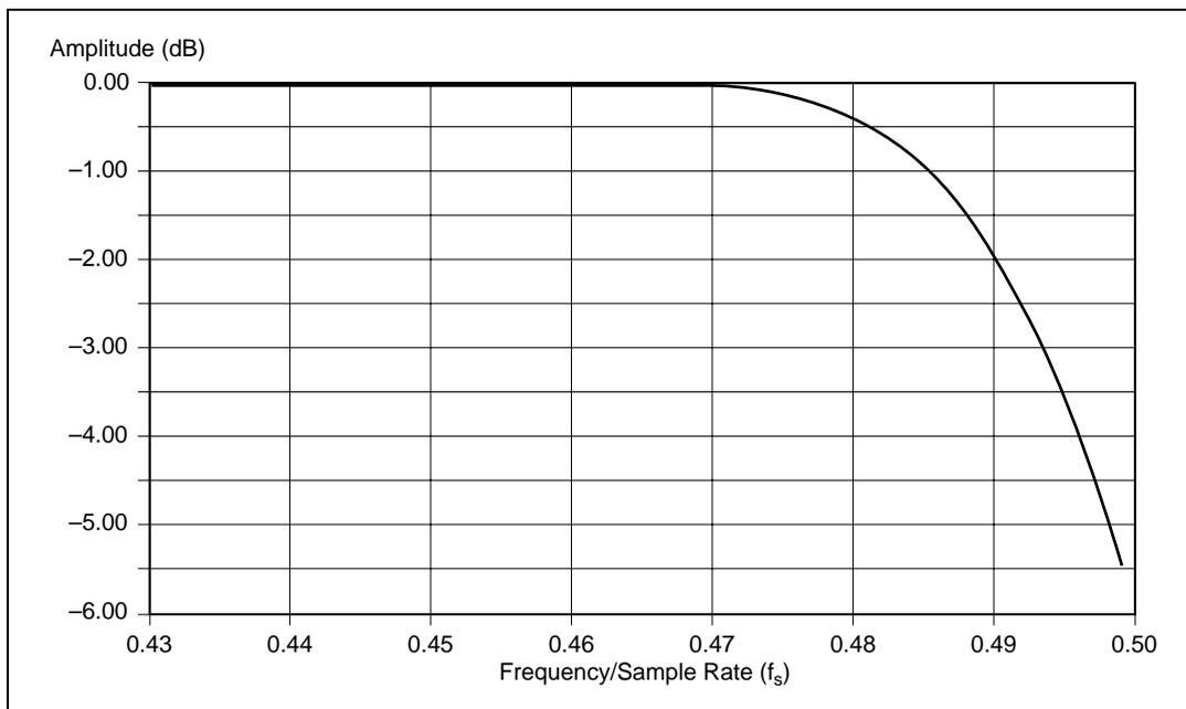
**Figure 6-2.** Input Frequency Response Near the Cutoff
