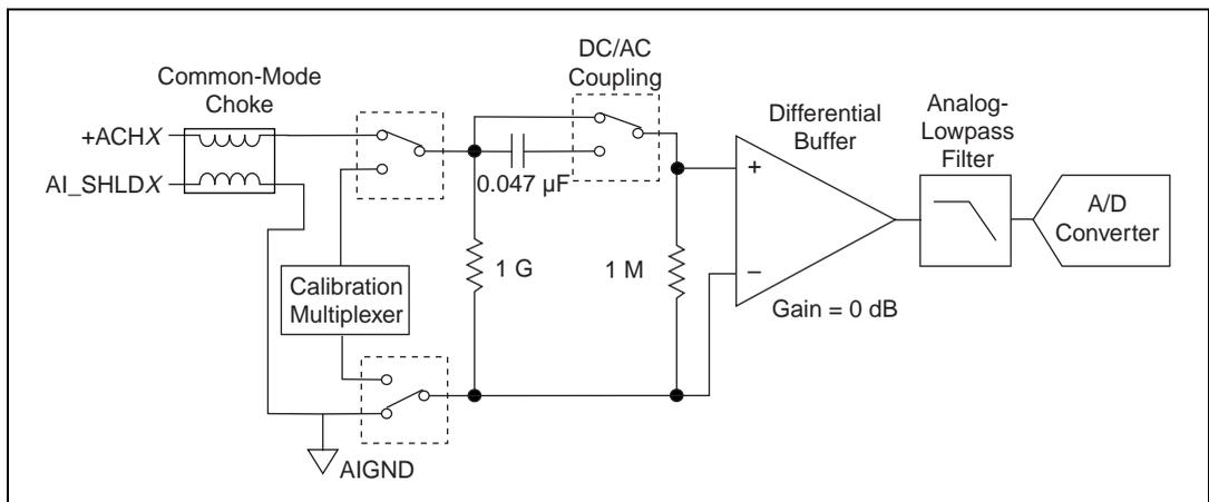
**Figure 4-5.** Analog Input Stage of the PCI-4453/4454
