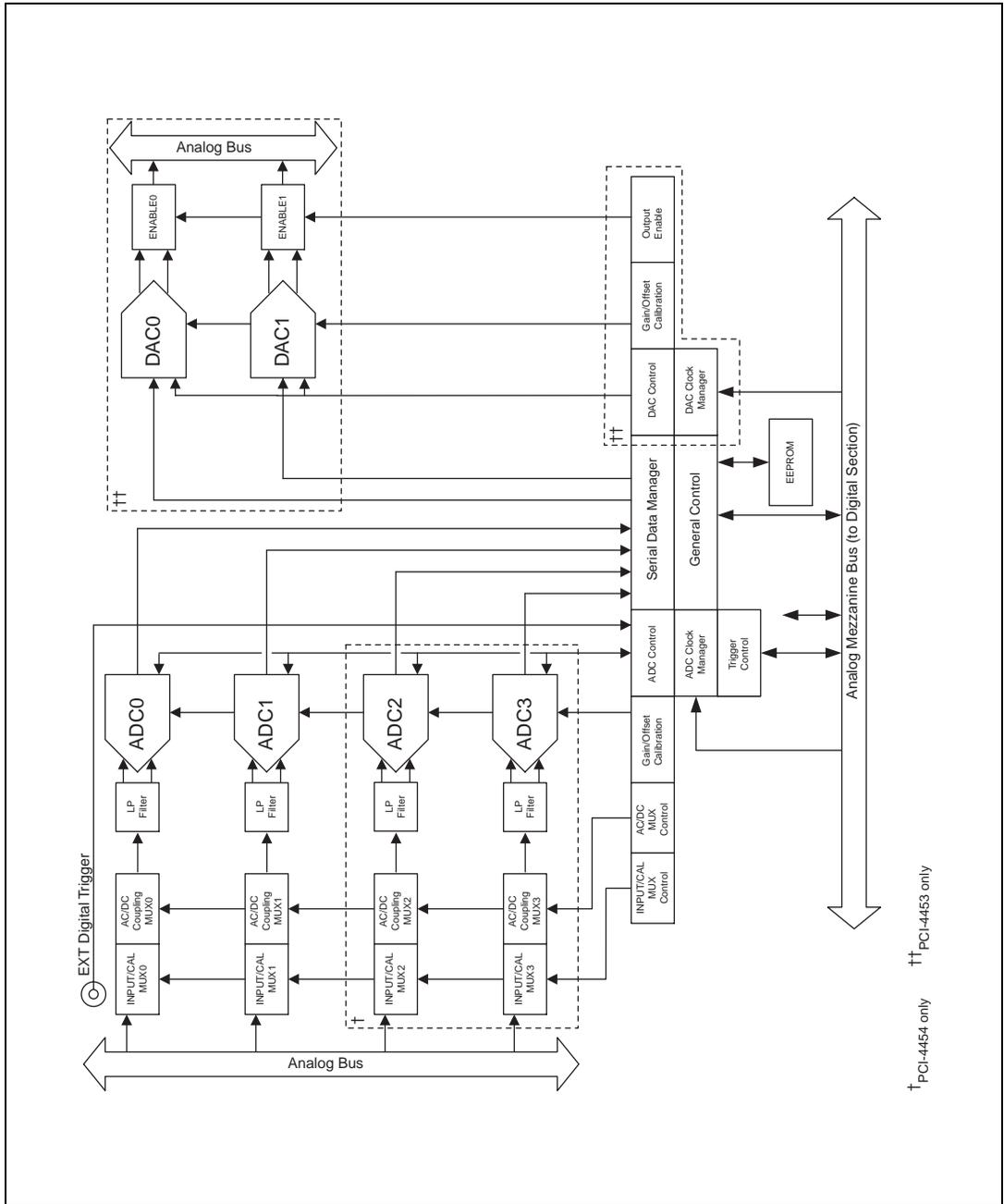
Figure 3-3. PCI-4453/4454 Analog Function Block Diagram
