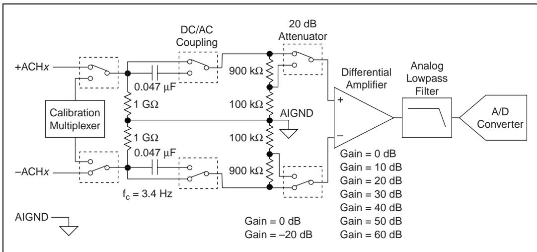
**Figure 4-4.** Analog Input Stage of the PCI-4451/4452
