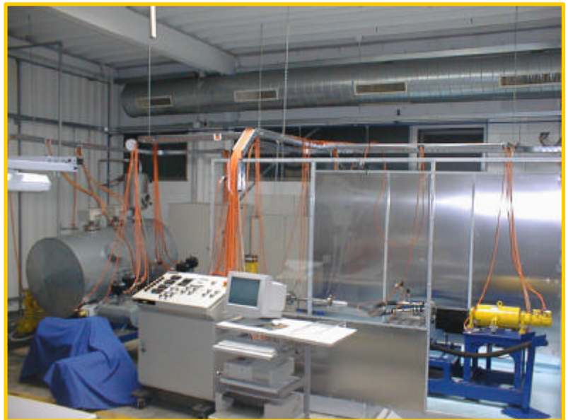
Picture 1 Automated Test Stand for Otto- and Diesel Engine Waterpumps
