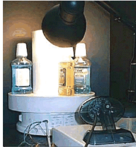
Fig. 1. Level gauging Station in HTTTL. Rotating table moves bottles across field of view.
