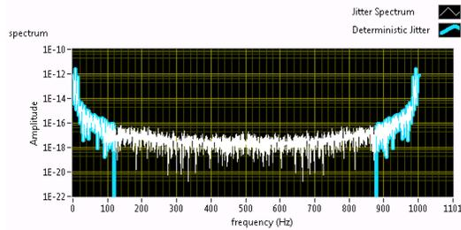
Figure 10. With the LabVIEW graphical development environment, you can enhance built-in graphs by programming them to go beyond just displaying the jitter spectrum. Figure 10 shows how you can use LabVIEW to highlight the signal's deterministic jitter components (in blue) with code from one of the toolkit's example programs.
