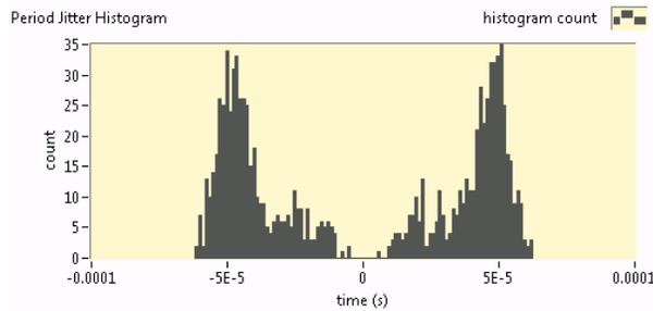
Figure 12. Histogram View of Period Jitter
