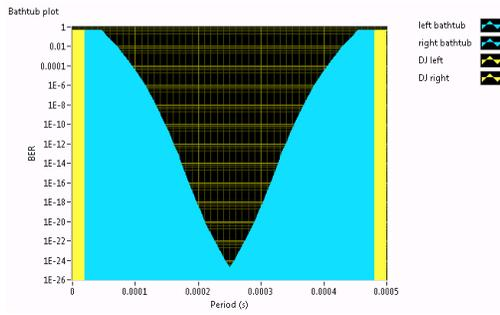
Figure 9. You can use the LabVIEW Jitter Analysis Toolkit Bath tub Plot Support VI to visually display eye opening as a function of bit error rate and provide insight into random and deterministic jitter.
