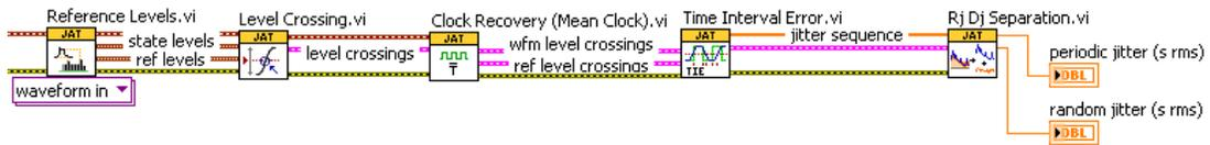
Figure 2. The typical jitter measurement workflow includes defining reference and state levels for the measurement, identifying level crossings in the signal, performing clock recovery (if required), calculating TIE, and measuring jitter components.
