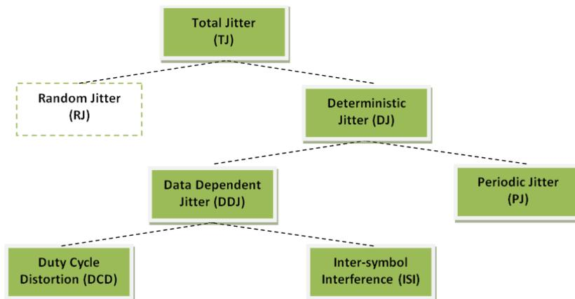
Figure 1. The NI LabVIEW Jitter Analysis Toolkit provides VIs for the measurement of TJ, DJ, DDJ, DCD, and PJ (solid boxes); RJ/DJ separation (dashed-line box) is included in the toolkit as an example program.
