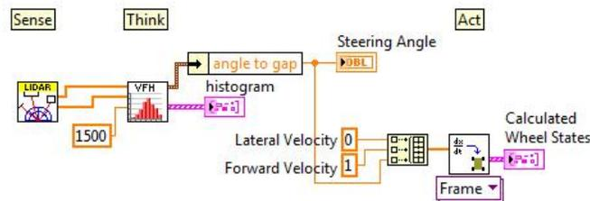
Figure 1. A Simple Behavior-Based Robot Program
