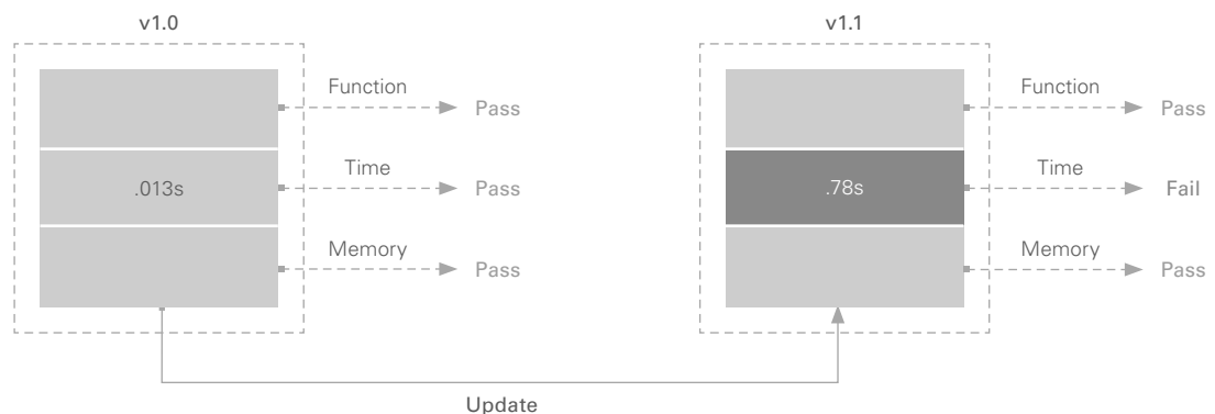
FIG 8 After performing a unit test of both the v1.0 and v1.1, the processing time is identified as a problem after the update, causing false failures in the process functional test.
