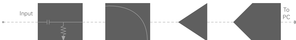
FIG 2 | Analog instrumentation input stages
