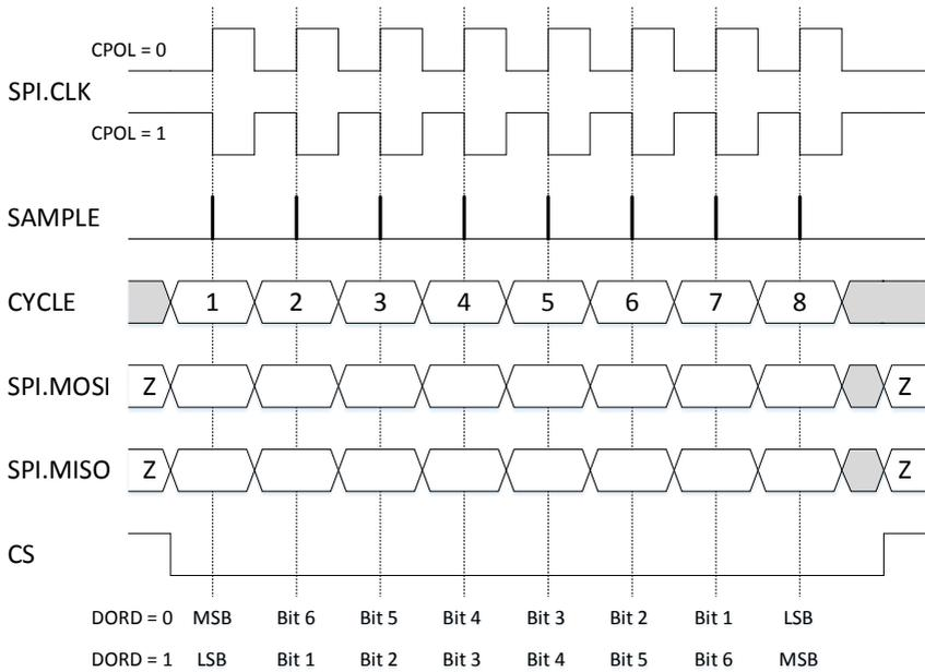
Figure 2. SPI Transfer Format with CPHA = 0
