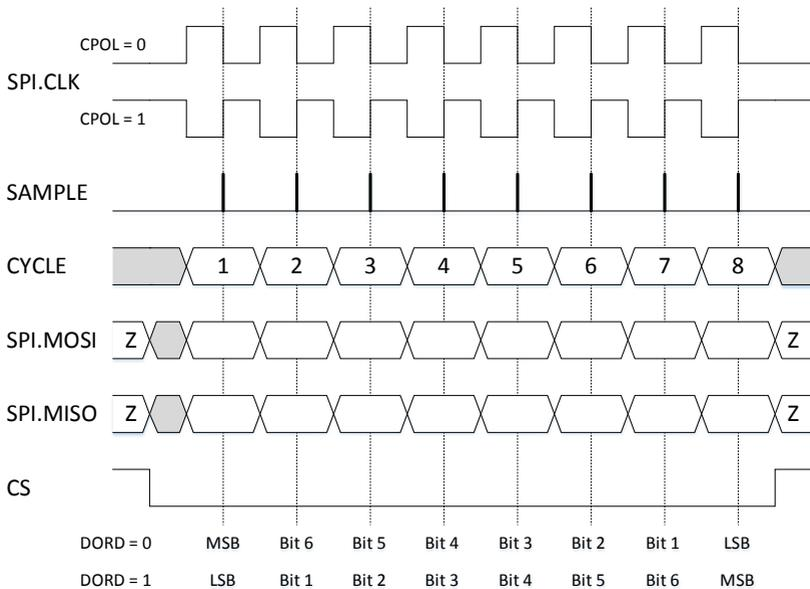
Figure 3. SPI Transfer Format with CPHA = 1
