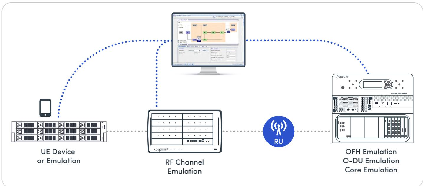
All the above is controlled by a single User Interface (UI) with access to power automation capabilities via RESTful or Tcl APIs.
