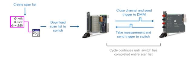
FIGURE 40 Depiction of the Scanning Process from the NI-SWITCH API to the DMM
