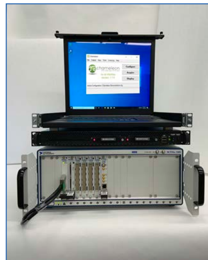
Rack-mounted monitor server with RAID & NI PXI chassis.
