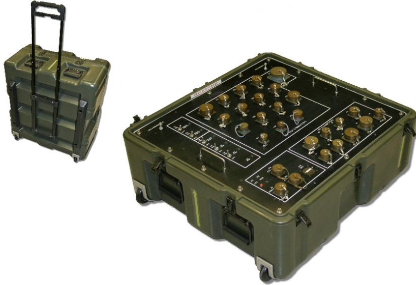
The CSU acts like a custom test and measurement instrument that can communicate to an MST Controller through an Ethernet connection. Specifically, the CSU has two standard RJ-45 ports allowing up to 2 MST Controllers to be connected to the CSU. Several of the LRUs have one or multiple static IP addresses.
