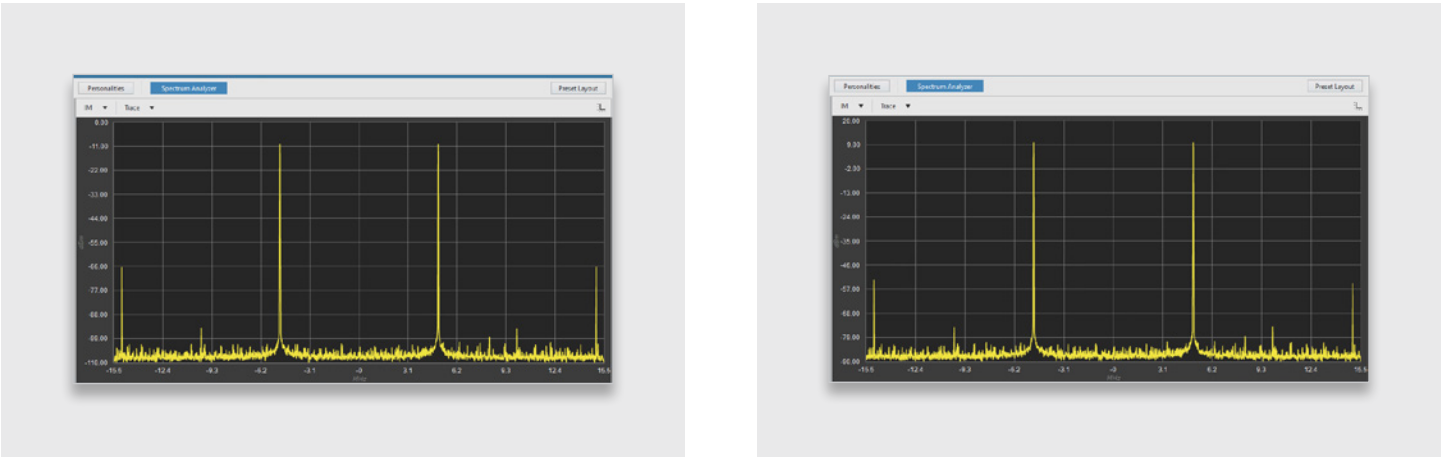
FIGURE 6 OIP3 Performance of Single Signal Source: -10 dBm (left) +10 dBm (right) per Tone, 10 MHz Spacing @ 5 GHz
