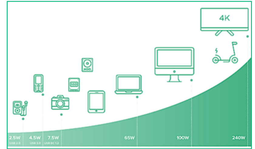
USB-PD 3.1 pushing past 100W
