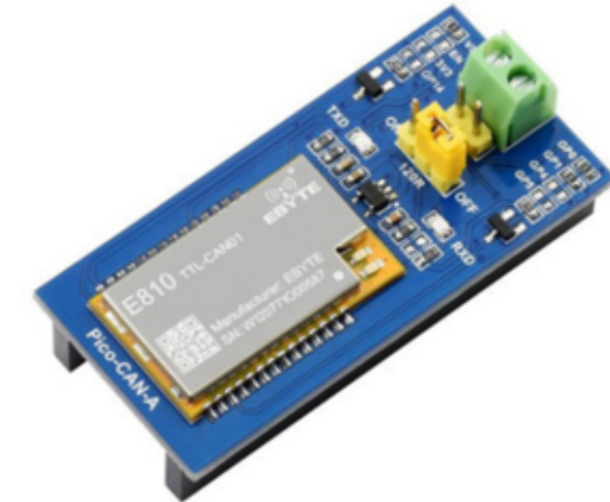
CAN Bus Module for Raspberry Pi Pico, UART to CAN conversion
