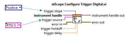
Configures the common properties of a digital trigger.
