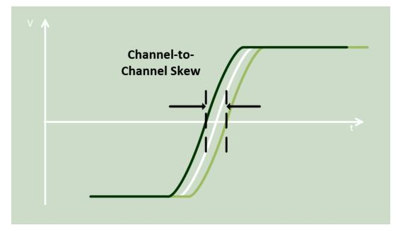
A clock or trigger, sent by the same source, may become unaligned by the time it reaches two different destinations.
