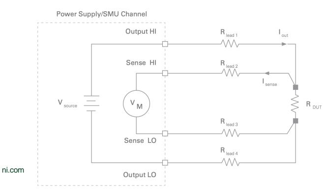
$R_{force} = R_{DUT} + R_{lead1} + R_{lead4} = 12\Omega$
