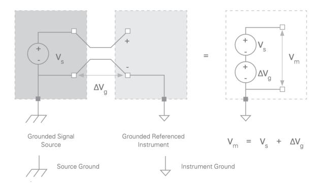
Ground loops can affect shielded differential measurements
