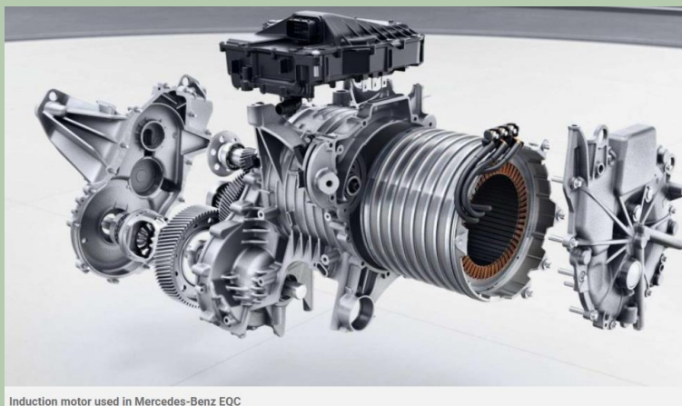
Induction motor used in Mercedes-Benz EQC
