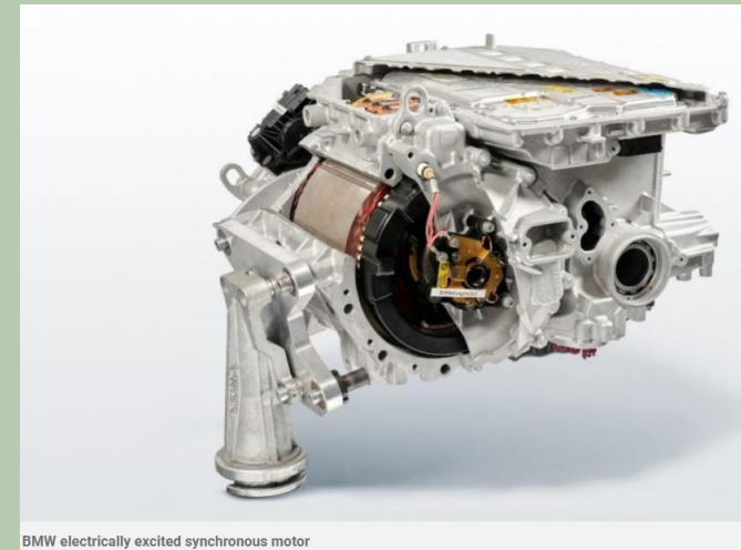
BMW electrically excited synchronous motor
