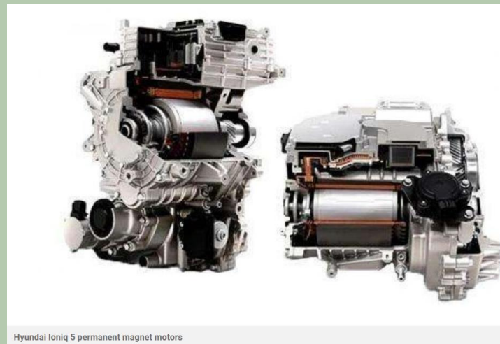
Hyundai Ioniq 5 permanent magnet motors
