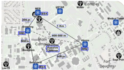
POWDER PAWR platform. ID BSs transmitting 5G/LTE/WiFi waveforms
