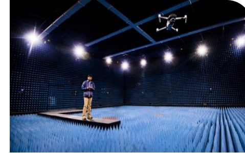
Using ensemble of classifiers with data collected in RF anechoic chamber
