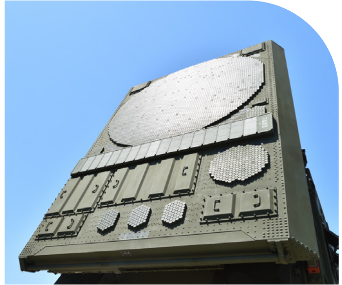
FIG 2 | An AN/MPQ-53 Ground-Based Radar System Based on a Modern Passive Electronically Scanned Array (PESA) Architecture
