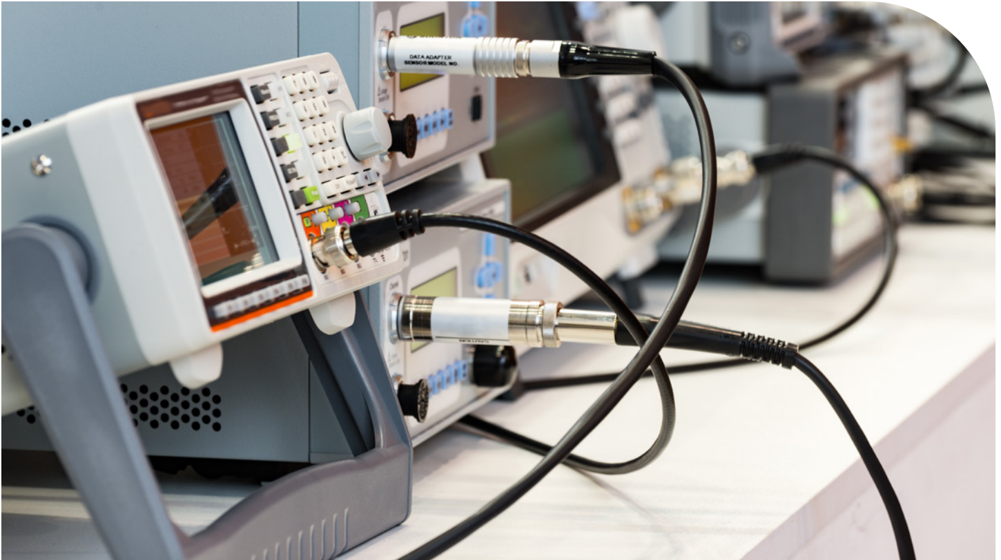
FIG 7 | A typical validation bench or automated test system includes a wide variety of RF, DC, and digital instrumentation. Depending on specific capabilities, vendor compatibility, and software control, integration of the various instruments into a cohesive test system can be challenging.
