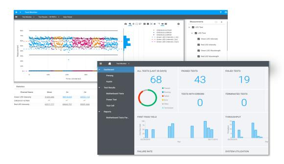
FIGURE 11. Dashboards built with SystemLink software help monitor test-station status and high-level data output.
