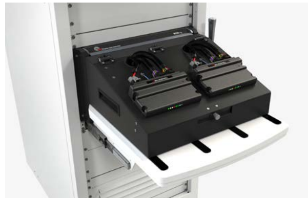
FIGURE 07 VPC 9025 TR with Fixture and DUTs
