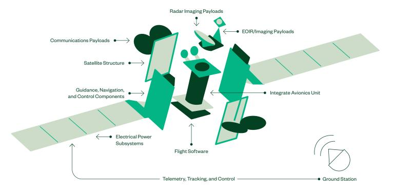
$Satellites\ are\ composed\ of\ various\ sensors,\ avionics\ subsystems,\ power\ electronics,\ communication\ systems,\ and\ a\ unique\ mission\ payload.$
