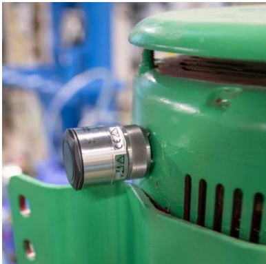
Wireless Vibration Sensor Monitoring an Electric Motor for a Pump
