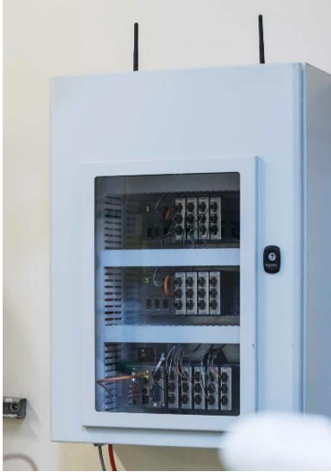
Wireless Access Point Connects Wired I/O to Wi-Fi Source: National Instruments
