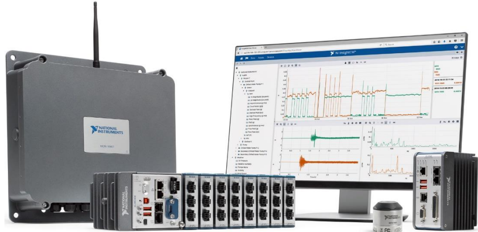
Example platform – InsightCM - that uses IoT technologies including edge processing, MEMS sensors, BLE5 wireless communication, and cloud/server/client connectivity protocols
