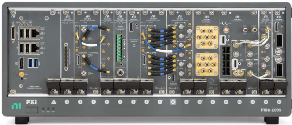
FIGURE 3 NI offers PXI modules for generating and measuring signals, with chassis options featuring up to 18 slots.
