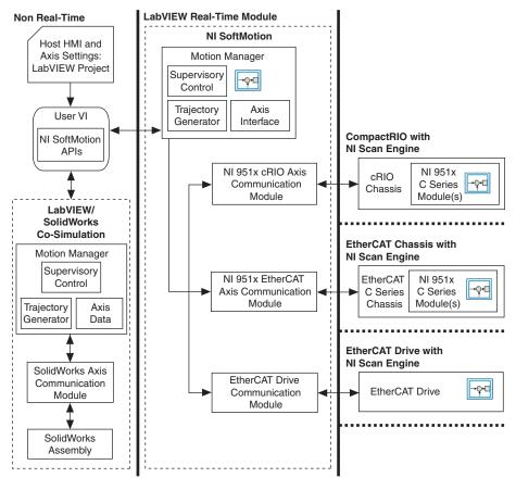
Figure 1. NI SoftMotion Module with SolidWorks and Hardware
