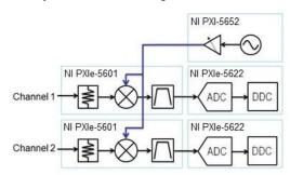
Figure 3. Synchronization of a Two-Channel Vector Signal Analyzer System
