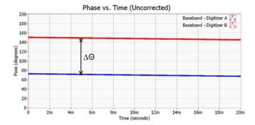
Figure 8. Each simultaneously sampled ADC has a constant phase offset.
