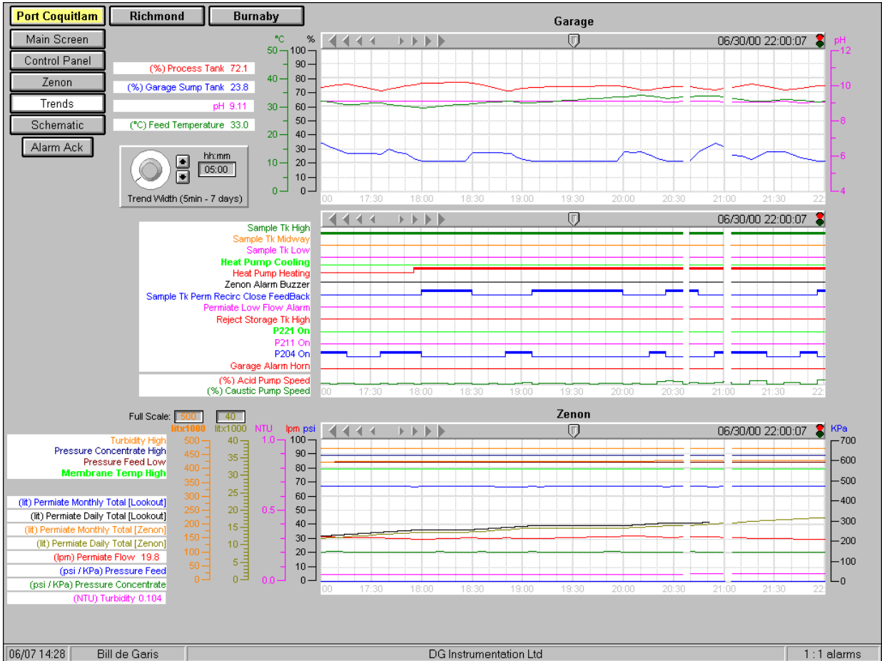
Figure 8. HyperTrends are used in this British Columbia transit water application in Canada. The HyperTrends are used to see real-time and historical data from the various pump flows in the application.
