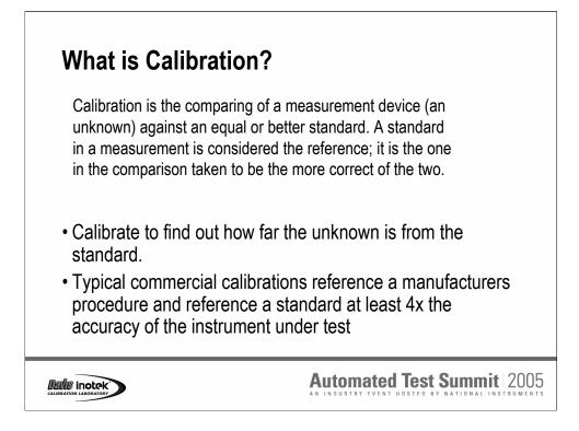
**Definition**: Calibration is the comparing of a measurement device (an unknown) against and equal or better standard. A standard in a measurement is considered the reference; it is the one in the comparison taken to be the more correct of the two. One calibrates to find out how far the unknown is from the standard.
