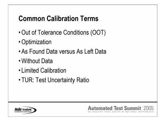
**Out of Tolerance Conditions**—If the results are outside of the instrument's performance specifications it is considered an OOT (Out of Tolerance) condition and will result in the need to adjust the instrument back into specification.
