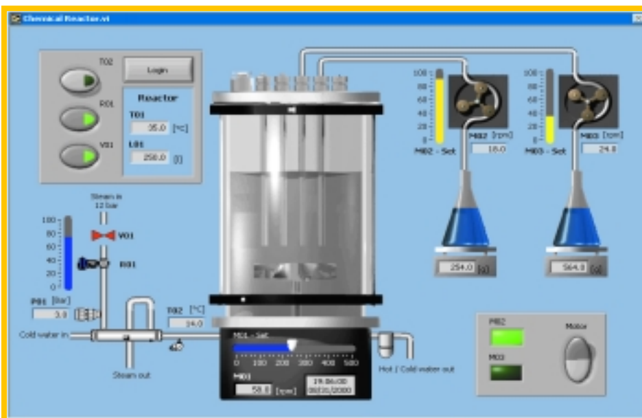
Chemical Reactor Application Using LabVIEW Datalogging and Supervisory Control Module
