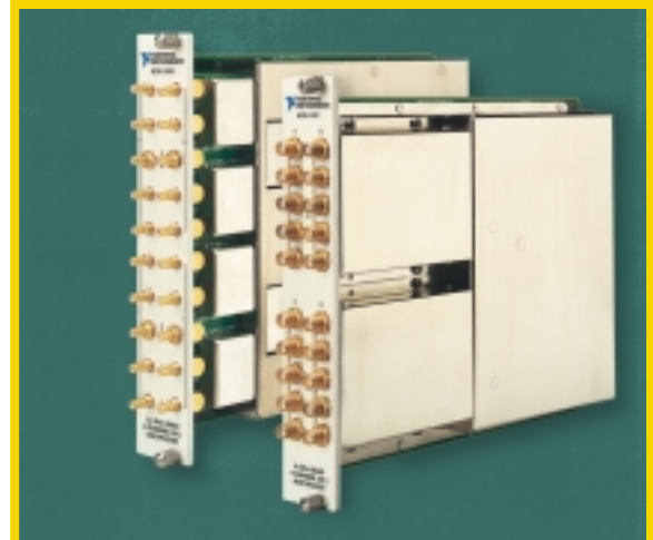
Use SCXI-1190 and SCXI-1191 for high-frequency applications.
