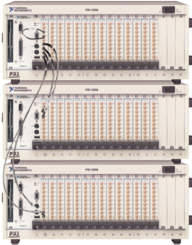
Figure 5. In this example, three PXI chassis containing 13 PXI-4472 8-channel 102.4 kS/s simultaneous-sampling dynamic signal acquisition modules are synchronized. The result is a 312-channel synchronized acquisition system.
