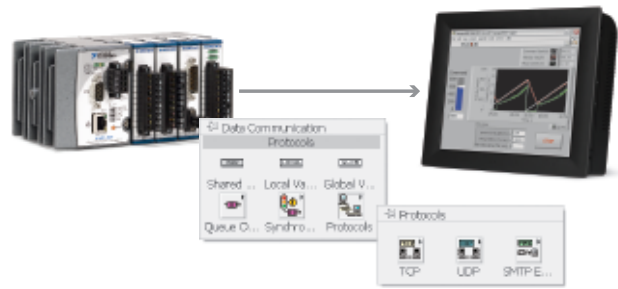
Figure 6. Standard TCP/IP Communication with Native LabVIEW TCP/IP VIs
