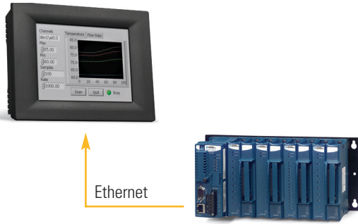
Figure 4. Touch Panel Display for Compact FieldPoint Connected over Ethernet
