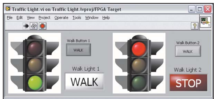
Figure 1. Interactive Front Panel of a Traffic Light Design Implemented on the NI Digital Electronics FPGA Board
