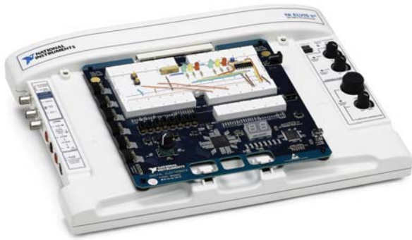
Figure 2. NI Digital Electronics FPGA Board Plugged into NI ELVIS II
