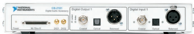
Figure 3. The NI CB-2181 digital audio accessory provides one digital audio input channel and one digital audio output channel. Each channel has a software-selectable BNC, TOSLINK, or XLR connection.
