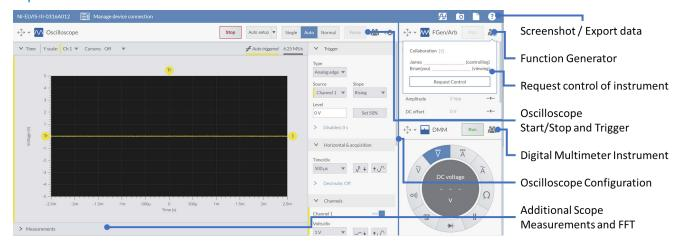
Figure 6. NI ELVIS III Oscilloscope Soft Front Panel
