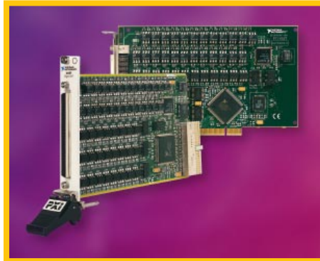
NI 6527 devices have 48 bits of isolated digital I/O.
